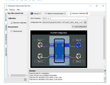
The AITT VNA Control allows a user to control a VNA to perform calibration and measurements locally or remotely from a separate PC by simply entering a 127.0.0.1 or the VNA IP address, respectively.
