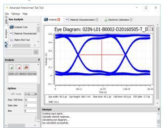
The AITT Analysis tool enables an engineer to perform frequency-domain, time-domain, and eye-diagram analysis. Its powerful plot tools make comparing data of different measurements easy.
