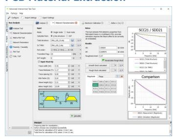
The AITT-ME material extraction tool extracts DK, DF, and surface roughness of a PCB from trace measurements based on the Huray roughness model. It supports single-mode and dual-mode data.
