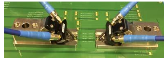
40/20 GHz Delta-L+ Handheld Probes
