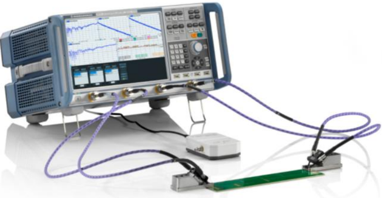
R&S®ZNB40 setup with Delta-L 4.0 probes
