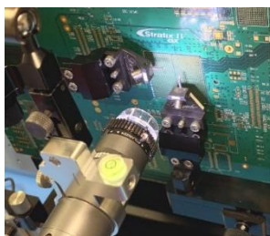
MA02 holds the microscope perpendicularly to PCB
