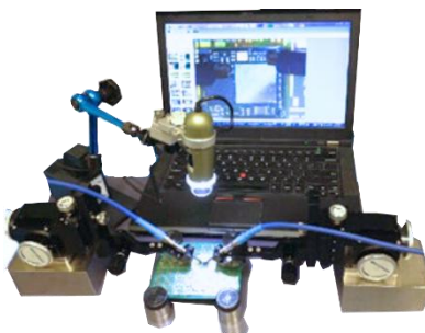
Horizontal probing of RF Module
