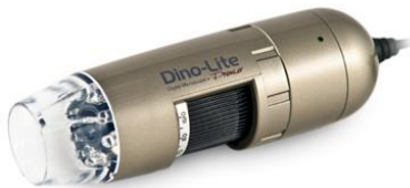
USB Digital Microscope (~ 90 x magnification)
