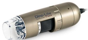
USB Digital Microscope (~ 90 x magnification)
