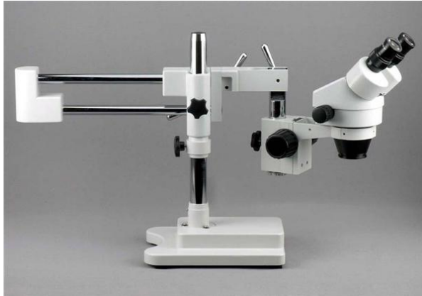
Optical Microscope (~ 90 x magnification)
