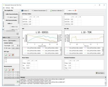
The Delta-L+ PCB characterization application offers the complete 1L, 2L, and 3L analysis based on Intel's Delta-L+ methodology. It guides the user to take measurements and perform analysis.
